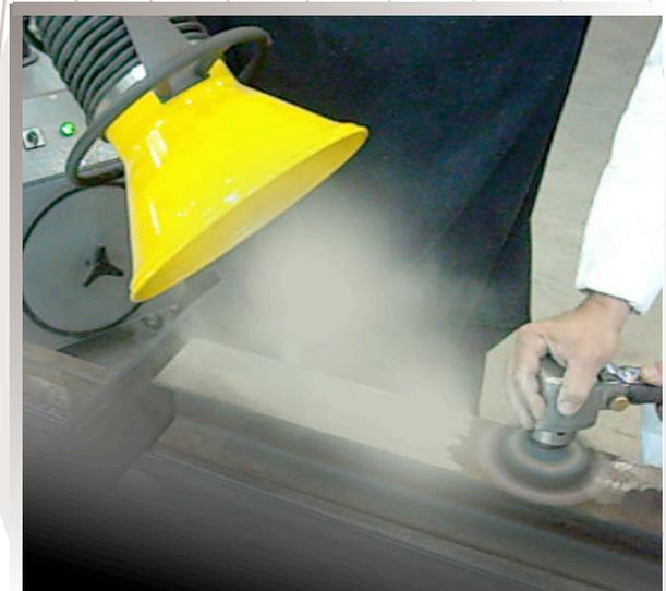
*Safety note : units are not designed to collect possible explosive dusts such as aluminum, magnesium, wood chips or similar. Refer to **ASHRAE** industrial ventilation handbook for references. If used for such applications, it is highly recommended to empty dust collector drawers in units between applications. **DO NOT MIX COLLECTION OF EXPLOSIVE DUSTS IN UNITS.***
